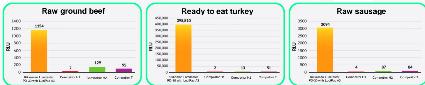
Figure 1: Comparison of the detection of RLU levels in meat (raw minced beef, raw sausage, and turkey) with A3 technology and conventional ATP test devices (Kikkoman Biochemifa Company 2022).
